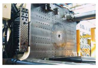
This multi coupler system for horizontal loading connects water and electric connections trouble free in less than 20 seconds. Another advantage of these multi couplers is that misconnections are being made any longer, which reduces the amount of bad products.
